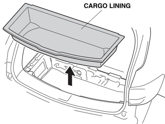
4. Locate and remove the rubber plug to access the spare tire hoist shaft. Lower the spare tire completely.
