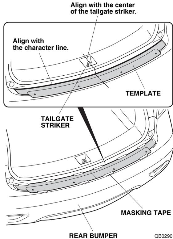
6. Using a pushpin, pierce four marks through the template as shown.
